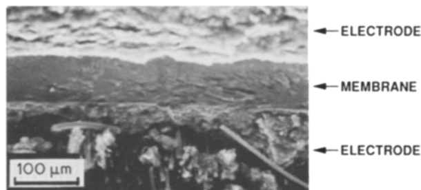
Fig. 4. SEM micrograph of cross-section of M&E assembly of the 20 wt % Pt/C electrode with sputtered layer of Pt (50 nm).
